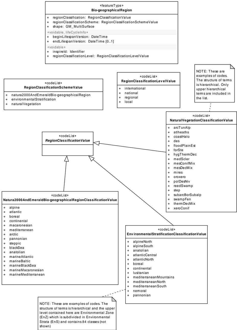
**Figure 4 – UML class diagram: Overview of the *Bio-geographical Regions* application schema**
