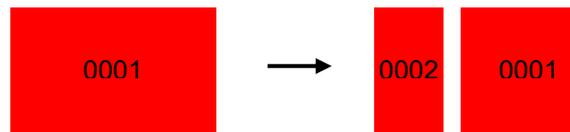
**Figure 26 – Application of the splitting rule. The area of the small new spatial object is less than 50% of the area of the original spatial object. It doesn't take over the TOP10\_ID but gets a new TOP10\_ID. The area of the large new spatial object is more than 50% of the surface of original spatial object and takes over the TOP10\_ID 0001.**
