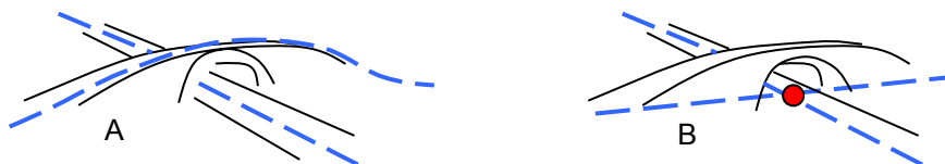
Figure 8 – Example A is a network only with nodes at level crossings and example B a planar network with a node in the crossing. This node will be complemented with the information separated crossing
